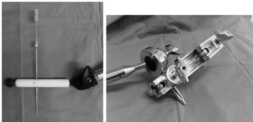
FIG. 2. Needle arrangement using 10-gauge metal guide on the device, a 14F metal "liver biopsy" needle, and an 18F, 20 cm "two part disposable needle" (left). The bracket to attach to a metal right angle (anesthetic screen) is to be secured to the operating table (right).
