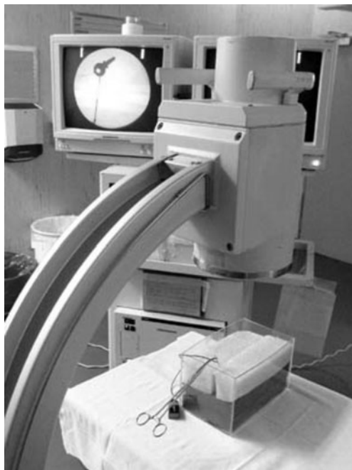
FIG. 5. In vitro testing using simulated fluoroscopy puncture with a small (2 cm) hidden radiopaque key connected to an electric circuit to indicate when the key is touched by the puncture needle.
