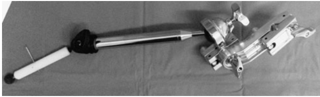
FIG. 1. The percutaneous nephrolithotomy navigation apparatus consists of a metal bracket (right) that is secured to a metal anesthetic screen. It has two adjustable and lockable multidirectional heads and a radiolucent end piece (left) that contains the metal guide for "bull's-eye sign" fluoroscopic alignment.
