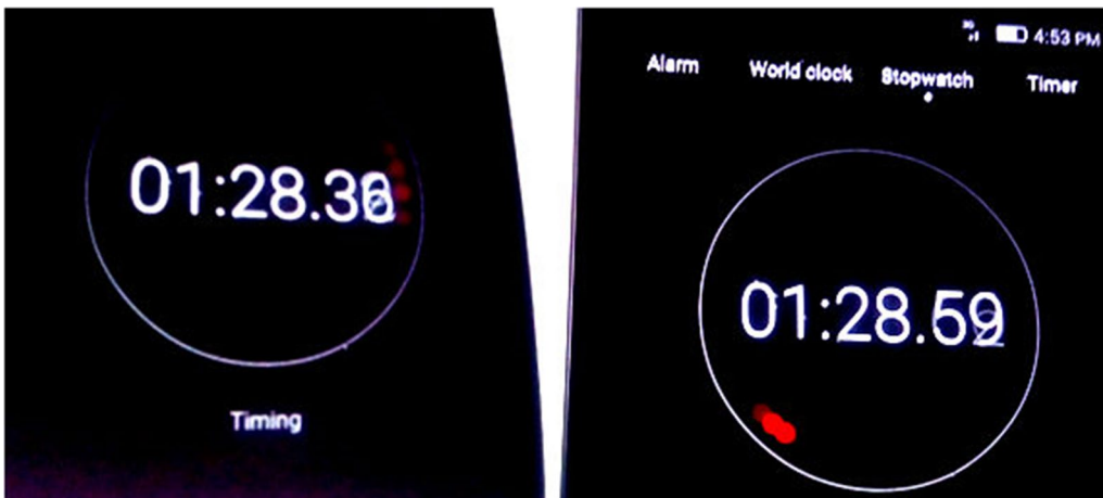
Fig. 4 Near real-time wireless video transmission with a virtually imperceptible latency of 200 ms. Left above is photograph of mobile phone stopwatch, and right image is photograph of computer monitor with wireless transmission from camera
