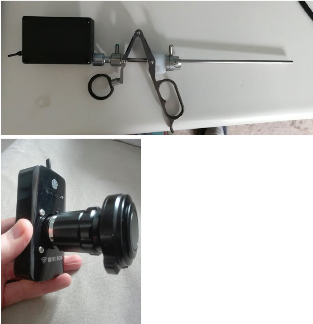
Fig. 3: 4 mm wireless cystoscope camera attached to a working element of a resectoscope (top). Wireless camera with optical coupler
