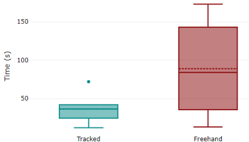
Figure 4: Comparison of mean simulated tracked ultrasound PCNL puncture (36 seconds) vs manual freehand PCNL puncture time (89 seconds), p=0.045 .
